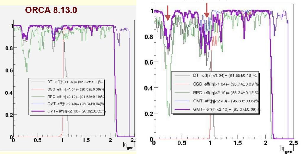
Larger inefficiencies in the central wheel crack and barrel/endcap overlap
